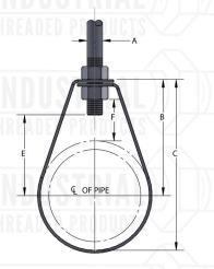
"E" dimension includes exposed rod threads beyond bottom of the hex nut. Exposed rod thread dimension is equal to the diameter of the rod used.
