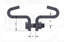
Material/Finish: Carbon steel ☐ 304 stainless steel ☐ 316 stainless steel Plain 🔲 electro-galvanized Service: Designed for attaching hanger rods from the center of an I-beam. Normally used with figure 26, 26W eyerods, or figure 13 weldless eye nut. **Approvals:** Complies with Federal Specifications WW-H-171-E (Type# 21), A-A-1192 A (Type# 21), and MSS SP-58 and SP-69 (Type# 21). Ordering: Specify clamp size, flange width, beam thickness, figure number and finish.
