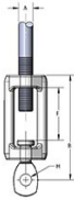
FIG. 114 - Page 93 TURNBUCKLE ADJUSTER WW-H-171-E TYPE 15 A-A-1192 A TYPE 15 MSS SP-58 and SP-69 TYPE 15
