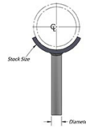
FIG. 420 - Page 106 PIPE SADDLE SUPPORT WW-H-171-E TYPE 37 A-A-1192 A TYPE 36 MSS SP-58 and SP-69 TYPE 36
