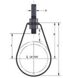
FIG. 31 - Page 30 ADJUSTABLE BAND HANGER WW-H-171-E TYPE 7 A-A-1192 A TYPE 7 MSS SP-58 and SP-69 TYPE 7
