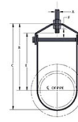
FIG. 11X - Page 19 CLEVIS HANGER WITH EXTENDED BOTTOM WW-H-171-E TYPE 1 A-A-1192 A TYPE 1 MSS SP-58 and SP-69 TYPE 1
