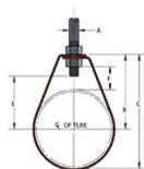
FIG. 31CT, 31CTI - Page 31 COPPER PLATED AND EPOXY COATED (COPPER-GARD), COPPER TUBING BAND HANGER WW-H-171-E TYPE 7 A-A-1192 A TYPE 7 MSS SP-58 and SP-69 TYPE 7
