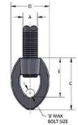
FIG. 47 - Page 80 EYE SOCKET WW-H-171-E TYPE 16 A-A-1192 A TYPE 16 MSS SP-58 and SP-69 TYPE 16
